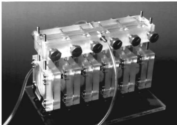
**Figure 11.** Six co-culture chambers, which are provided with aerobic and anaerobic gas mixtures via a joint supply system.
