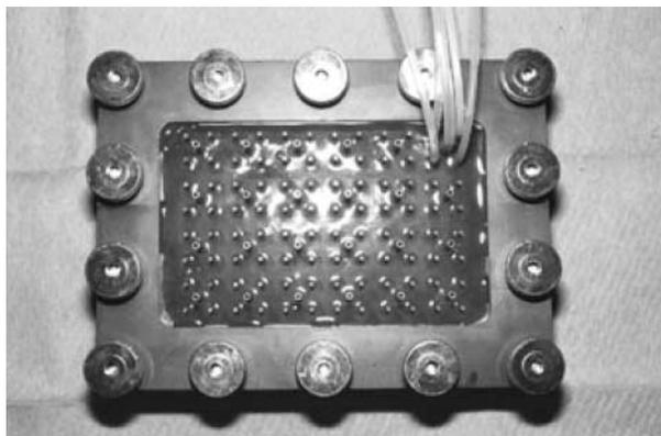
**Figure 16.** Mini bioreactor in 96-well format with perfusion system.
