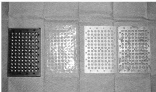
**Figure 15.** Scaffold, membrane, seal, and backing of metal as the components of 96-well mini bioreactor.
