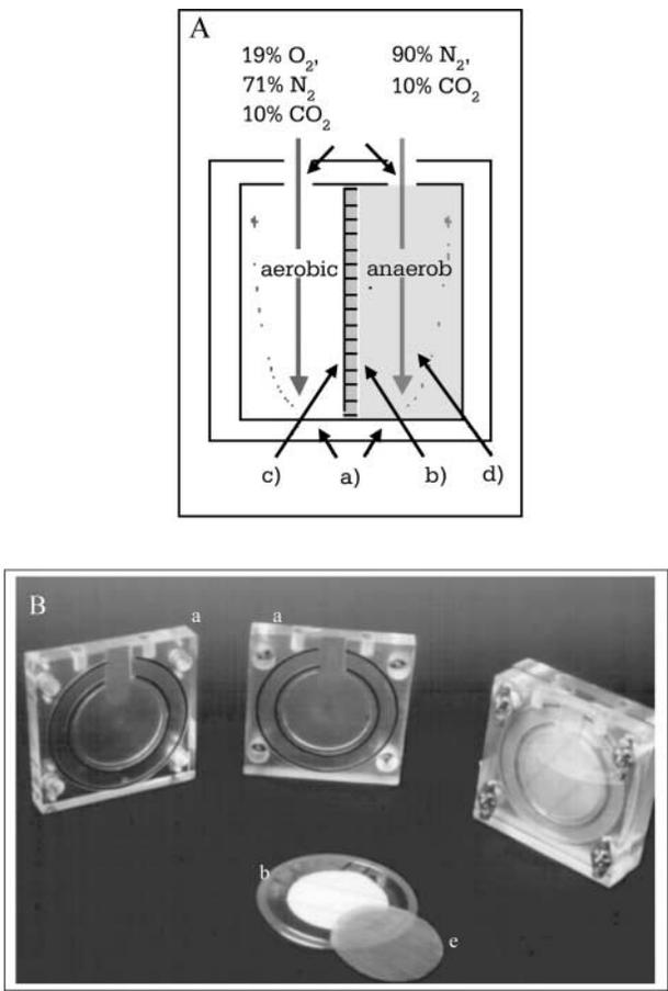
**Figure 10.** Schematic diagram (A) and photograph (B) of the two-chamber system: a) two halves of the device containing the culture compartments, b) polycarbonate membrane fixed between two tight-fitting rings, c) monolayer of hepatocytes, d) suspension of fecal microflora, e) a fine mesh for the protection of hepatocytes against gas bubbles, and f) cannulas for gassing the media project into each chamber.
